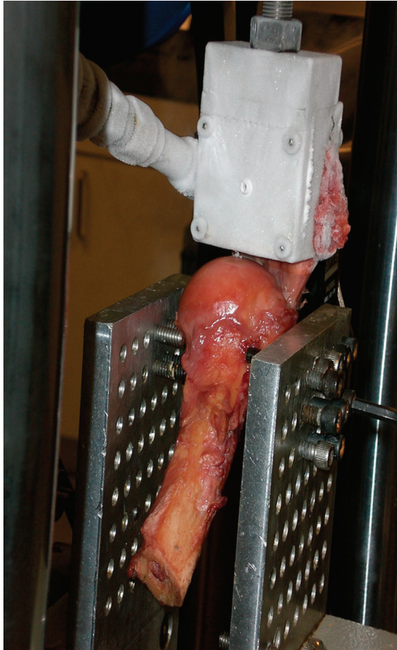
Fig. 7 Photograph showing the humeral head with rotator cuff tendons affixed to the liquid nitrogen freeze-clamp.
